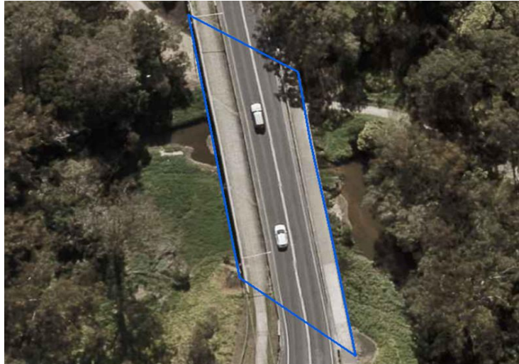
Figure 26 – Example of a Bridge extent envelope
